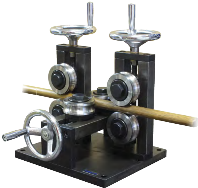
C 80-HWSY-2 Max Product Ø: 27mm Roller Ø: 80mm Article: 5933 Weight: 40kg
